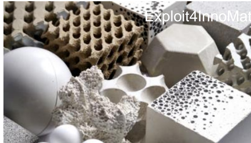
Lightweight graded concrete with lower CO 2 -footprint, ©ILEK
