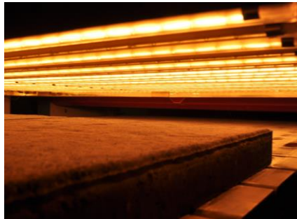
Drying of stone plates
